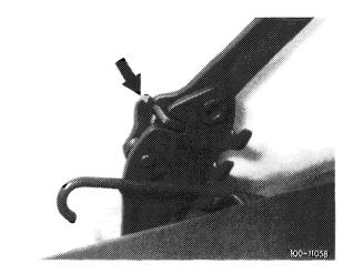
3 On engine 617, remove adapter at air cleaner (arrow).
