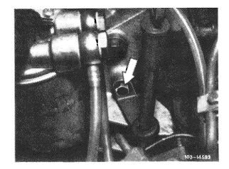
7 Release and remove V-belt of Delco refrigeration compressor.
