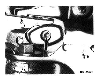
20 Attach hoist rope to suspension lug at front of cylinder head (arrow).
