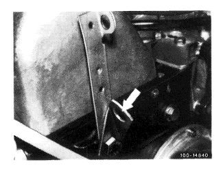
21 Using hoist and crane, raise engine until upper part of oil pan can be removed.
