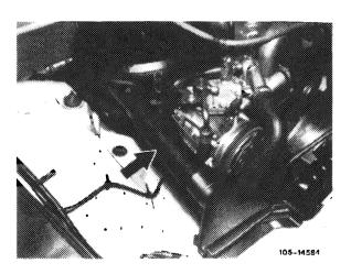
4 If model features uprated engine, also remove longitudinal control spindle. Unhook control rods for this purpose. Withdraw retainer (arrow) and force longitudinal control spindle in aft direction.
