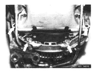
17 Using 9 mm diameter remover for valve guides, force out oil dipstick guide tube as far as possible.
