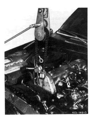
To remove oil pan, turn crankshaft with tool combination until upper part of oil pan can be drawn out beneath the connecting rods and crankshaft webs.
